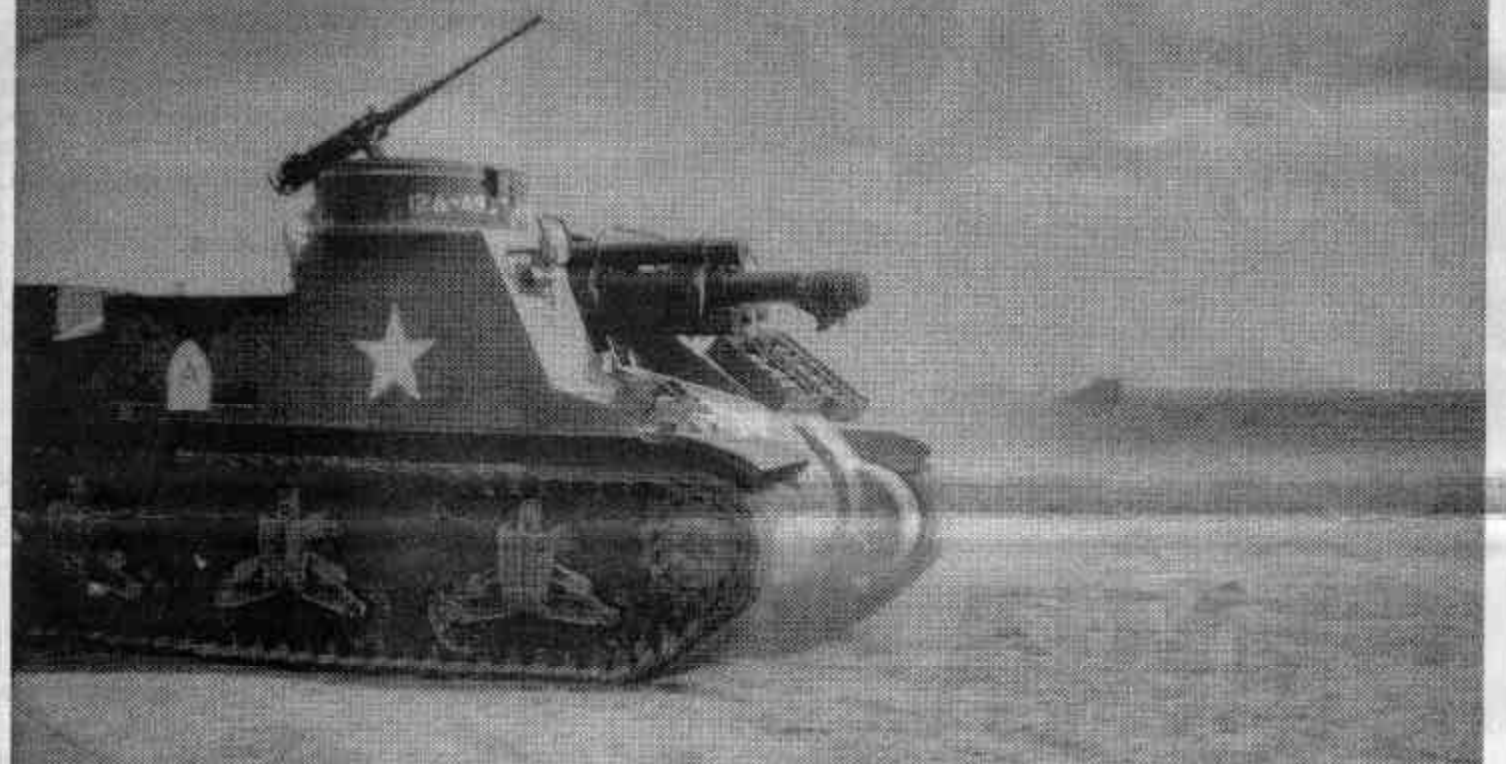
May 1944. The 12th Armored Division in training exercises in Texas. The vehicle pictured is an M7, self-propelled artillery.
